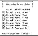
Once the configuration is complete switch **SW2 MUST** be switched to the ON position to apply the new settings. **SW2 MUST** remain in the ON position to use the new settings. Switch **SW2** back to OFF position to reset to the default settings. SW1 can be used to change the normal open or the normal close contacts for all relays. SW1 set to the OFF position; normal open (default), SW1 set to the ON position; normal close.
