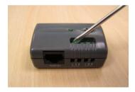
2. Connect the wires of SSL-DOOR to the SSL-EMD Alarm-1 and/or Alarm-2, and then tighten the screws.
