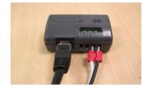
4. Verify that the SNMP-SSL card has a network connection and is powered on.
