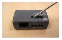
2. Connect the wires of SSL-WATER sensor to the SSL-EMD Alarm-1 and/or Alarm-2, and then tighten the screws.
