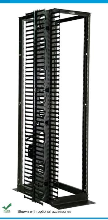
DIMENSIONS: 84"H x 20.6"W, Rail Depth Ranges from 24" to 36" RACK SPACES: 45 RMU • 19" EIA 310-D Compliant WEIGHT CAPACITY: 1500 lbs. when networked; 1000 lbs. free standing CONSTRUCTION: 12 Gauge Cold Rolled Steel and Extruded Aluminum SHIPPING WEIGHT: Please see Part No. Description
