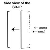
Attach the cover to the base with the two included screws as shown.
