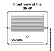
To open the speaker box, remove the two separate screws from the cover.
