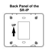
Mount back panel to a wall, a single gang box or a 4"x4" junction box with the arrow pointing up. **Note:** For outdoor applications apply a bead of caulk between back panel and wall.
