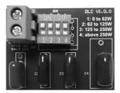
The VA-DLC dummy load capacitor is used for the speaker line surveillance based on impedance measurement. When a number of speakers are installed with long wires, the VA-DLC can provide a reliable monitoring method to detect the open circuit of entire speaker line even the last speaker.
