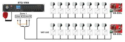
The VAT remote volume attenuator supports 2-wire connection and 3-wire connection, and is compatible with 100V and 70V loudspeaker lines.
